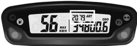
**ART function Accumulated Ride Time (screen 3):** displays the hours of operation of the vehicle.
