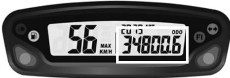
**ODO function Odometer (screen 3):** displays the total mileage traveled by the vehicle.
