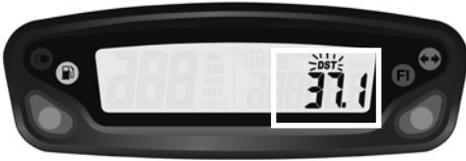
Fig 6 Adjustable trip distance function
